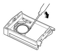
5. Put in the new battery (CR1620 or equivalent) with the positive pole (+ ) facing down.
